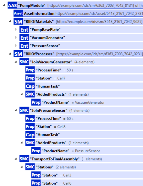
Figure 8: BoM and custom BoP submodels of a product subassembly in AASX Package Explorer.
